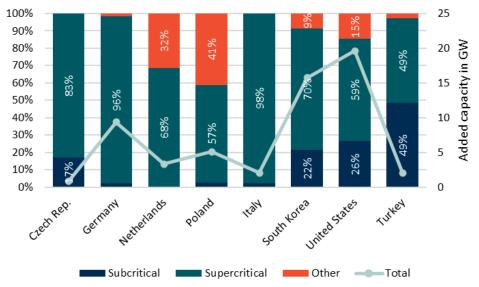
Figure 5-42 Technological structure of coal commissioning between 2008-2018: Selected Countries.
