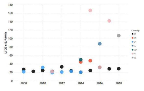
Figure 5-64 LCOE of Hydropower (Dam) power plants in selected countries
