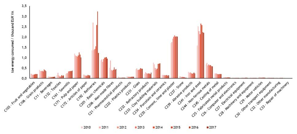
Figure 4-10 Energy intensities of industrial manufacturing sectors, 2010-2017, averages over limited number of EU Member States with available data
