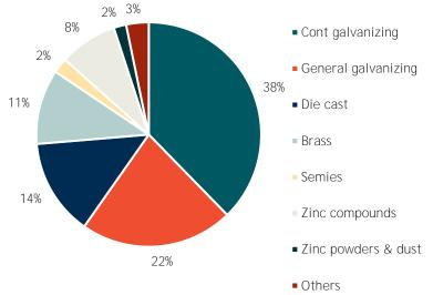
Figure D-19 Main usages of zinc - share of world-wide applications in tonnes.
